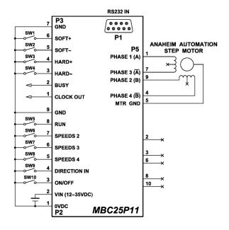
Power Requirements:12-35VDCOutput Current Range: $T_A = 25^{\circ}\text{C}$ <br/>0.5 - 2.5A PeakClock Out Frequency:77Hz - 15kHzDriver Chopping Frequency:25kHz - 30kHzOperating Temperature: $0^{\circ}\text{C}$  to  $70^{\circ}\text{C}$
